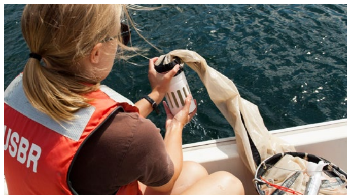
Reclamation conducts early detection sampling for invasive mussels using a plankton tow net at a Colorado Reservoir. (Reclamation)
